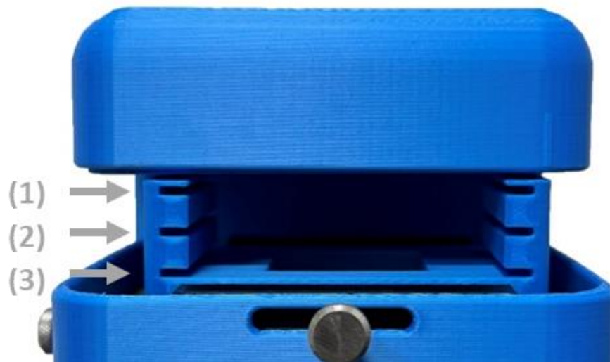
Figure 1. The face of the HoloScope, showing the three slots for sample mounting.
